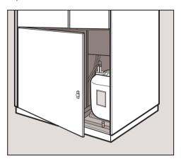
■ Open the service panel on the bottom right of the machine.
